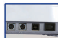
RS-232 interface for easy computer connectivity
